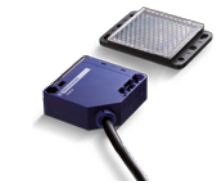
Extra 628 reflection light opto sensor • 24-240 V AC, 12-240 V DC, IP 54 • Range: 5 m • Can only be used as a pulse generator
